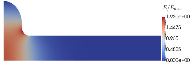
Figure 4: The electric field of the fundamental mode in half of the chosen RF cavity.
