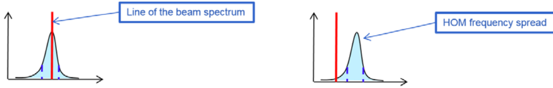
Figure 2: Stochastic HOM excitation by the pulsed beam. High excitation probability (left) corresponds to the case of the beam harmonic frequency within the HOM frequency spread and low probability (right) represents the beam spectrum line which is far off the HOM frequency deviation bandwidth.
