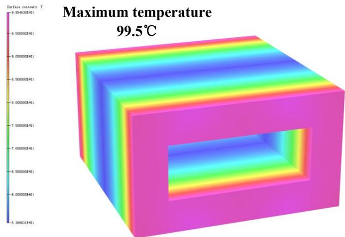
**(3)Temperature distributions of Laminations of iron core without slits**
