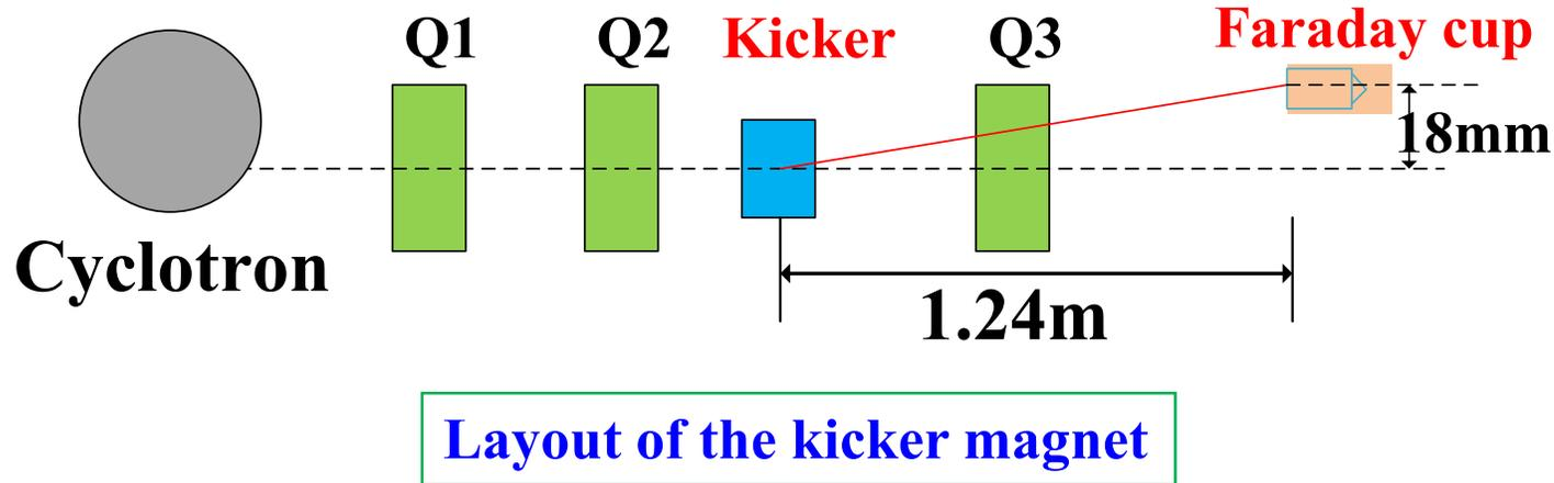
**Kicker magnet is located at 1.24m upstream of Faraday cup / beam stop. It switches ON/OFF the beam during spot scanning intervals and in safety situation.**
