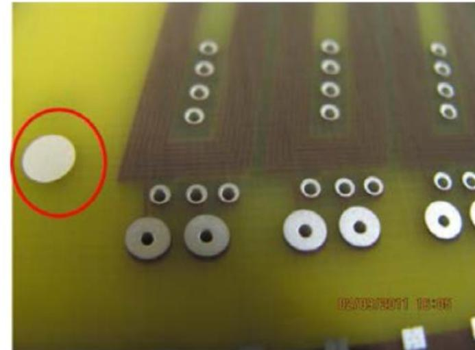
**A array searching coil made of PCB is now considered\*.**
