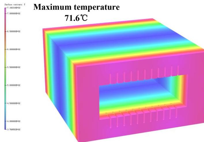
**(4)Temperature distributions of Laminations of iron core with slits**
