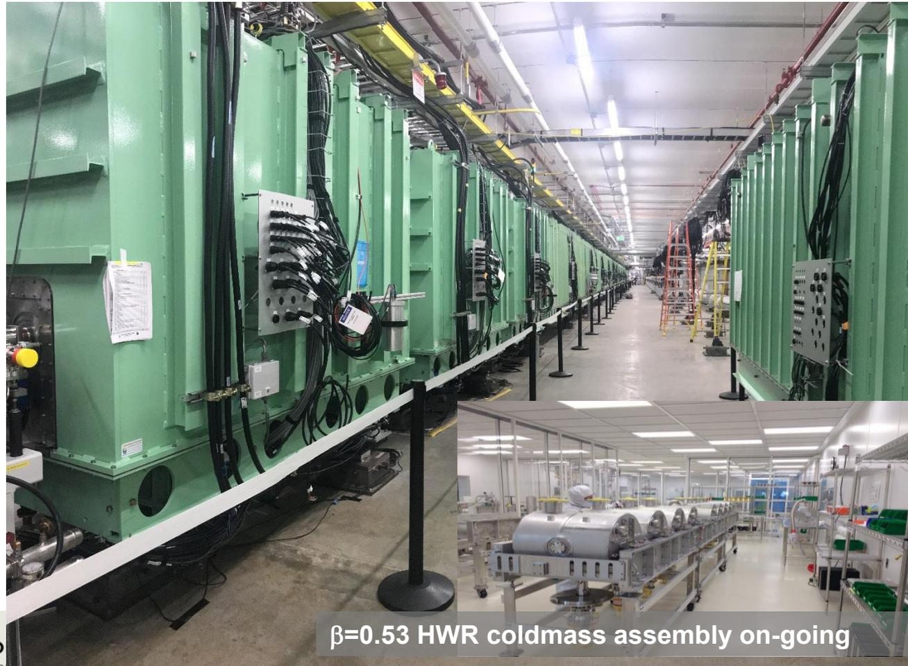
$\beta=0.53$  HWR coldmass assembly on-going
